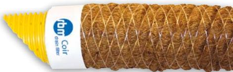
**Coir fiber 700 filter** | The O90 Test value of this filter is 700  $\mu\text{m}$  and holds back 90% of all soil particles bigger than 700  $\mu\text{m}$ . Coir fiber filters are degradable after a long time and have been successfully used in areas where a high quantity of iron ochre is in the ground.
