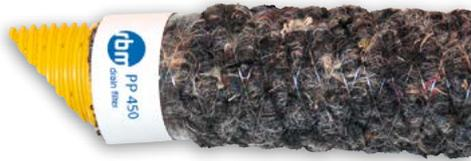
**PP 450 filter** | The O90 Test value of this filter is 450  $\mu\text{m}$  and holds back 90% of all soil particles bigger than 450  $\mu\text{m}$ . It consists of a blend of synthetic fibers and can be used for several soil types and circumstances and is manufactured according to the KOMO Standard.
