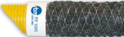
**PP 1000 filter** | The O90 Test value of this filter is 1000  $\mu\text{m}$  and holds back 90% of all soil particles bigger than 1000  $\mu\text{m}$ . The PP 1000 filter consists of coarse high class synthetic fibers and is a non degradable filter that is mainly used in soils with an high iron ochre content.
