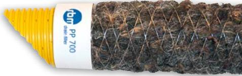
**PP 700 filter** | The O90 Test value of this filter is 700  $\mu\text{m}$  and holds back 90% of all soil particles bigger than 700  $\mu\text{m}$ . The PP 700 filter consists of a different blend of synthetic fibers than the PP 450 filter and is mainly used for loamy sands, sandy soils and peaty soils. It is manufactured according to the KOMO standard.
